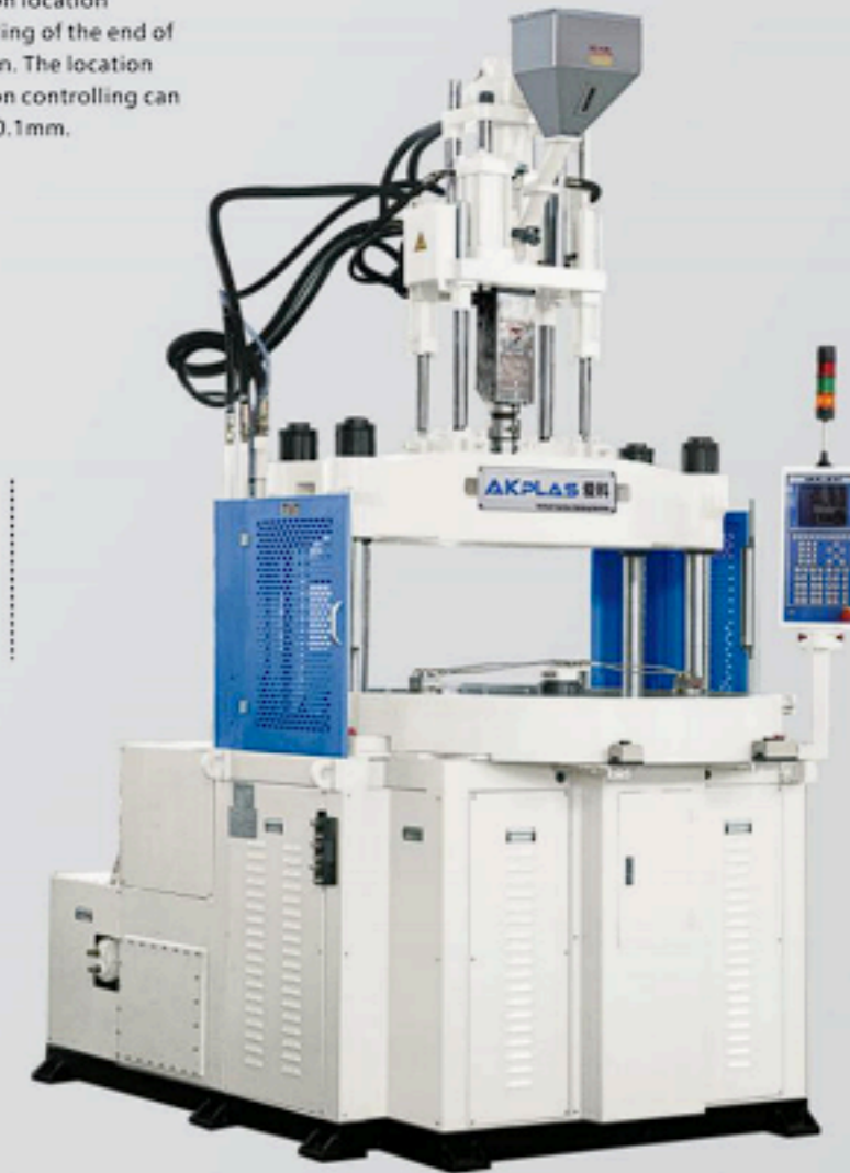
AT-2R Series 锁模力 35-450T Clamping Force 射出量 65-500g Shot Weight
